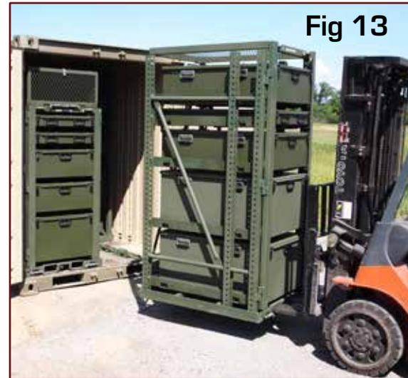
2. To remove the Removable Unit: Pull out the shot bolt(s) at the bottom releasing the unit. Using a qualified fork lift driver, the unit can be lifted out of the container with a forklift (Figure 13). An empty Half Width Removable Unit with drawers weighs approximately 1,000lbs, a full width removable unit with glide out shelves weighs approximately 1,500lbs
