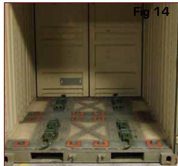
3. To replace the Removable Unit, move the unit over the Adapter Plate (Figure 14) until approximately centered. (Note: the shot bolt must be disengaged.) Lower the unit and it will self-center. Engage the shot bolts securing the Removable Unit.
